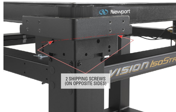
Figure 11: Shipping screw location – Each I-325A isolator has 2 shipping screws that will need to be removed in order to engage the horizontal leveling mechanism.
